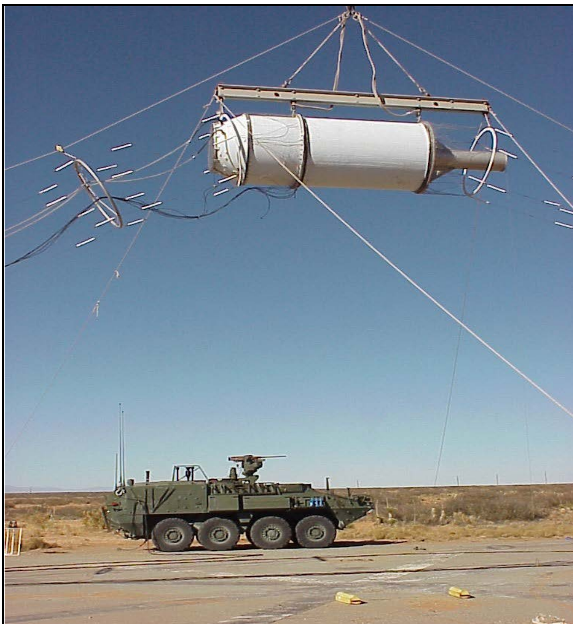
Figure C-1. Generic missile launcher HEMP test setup.
