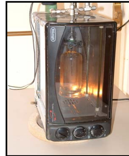
250 ml Confined Cook-Off Oven Assembly
