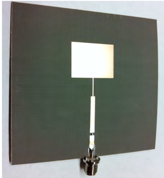
Figure 20: 5.5 GHz patch antenna with discrete reactive load
