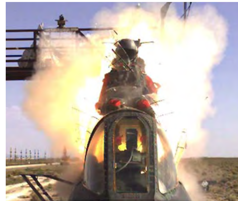
NSWC Indian Head specializes in Cartridge Actuated and Propulsion Actuated Devices (CADs & PADs) such as this Aircrew Escape Propulsion System (AEPS)
