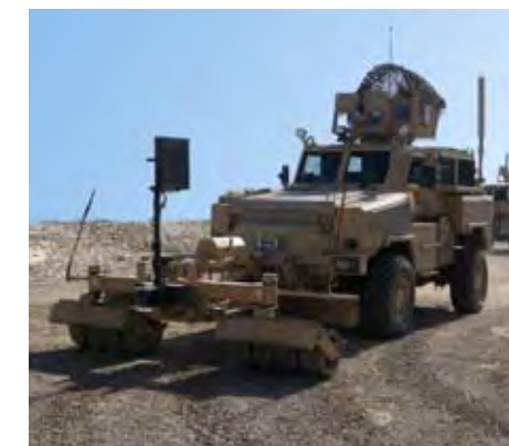
The SPARK mine roller system is meant to detonate improvised explosive devices before they can do serious damage to a vehicle and its occupants
