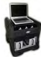
Environmental Sentinel Biomonitor (ESB) System Increment 1
