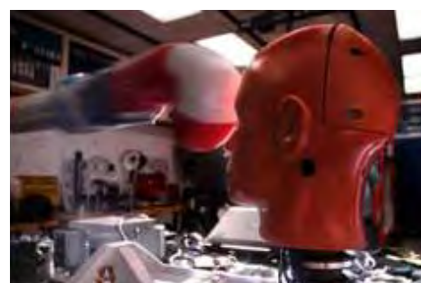
Blunt impacts to FOCUS are measured, and data is used to predict resulting eye and vision injuries
