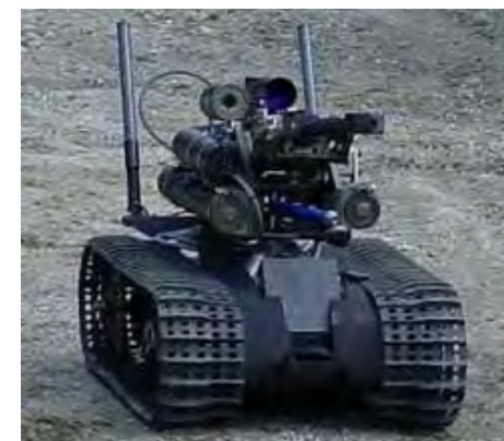
The TALON robot provides Soldiers the ability to identify explosive devices and mines visually and neutralize them from safe stand-off distances
