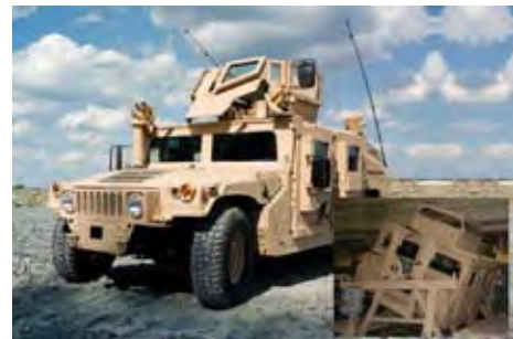
TARDEC's HEAT trains Soldiers how to react in vehicle rollover situations. The HEAT is pictured at bottom right in the inset of this up-armored humvee
