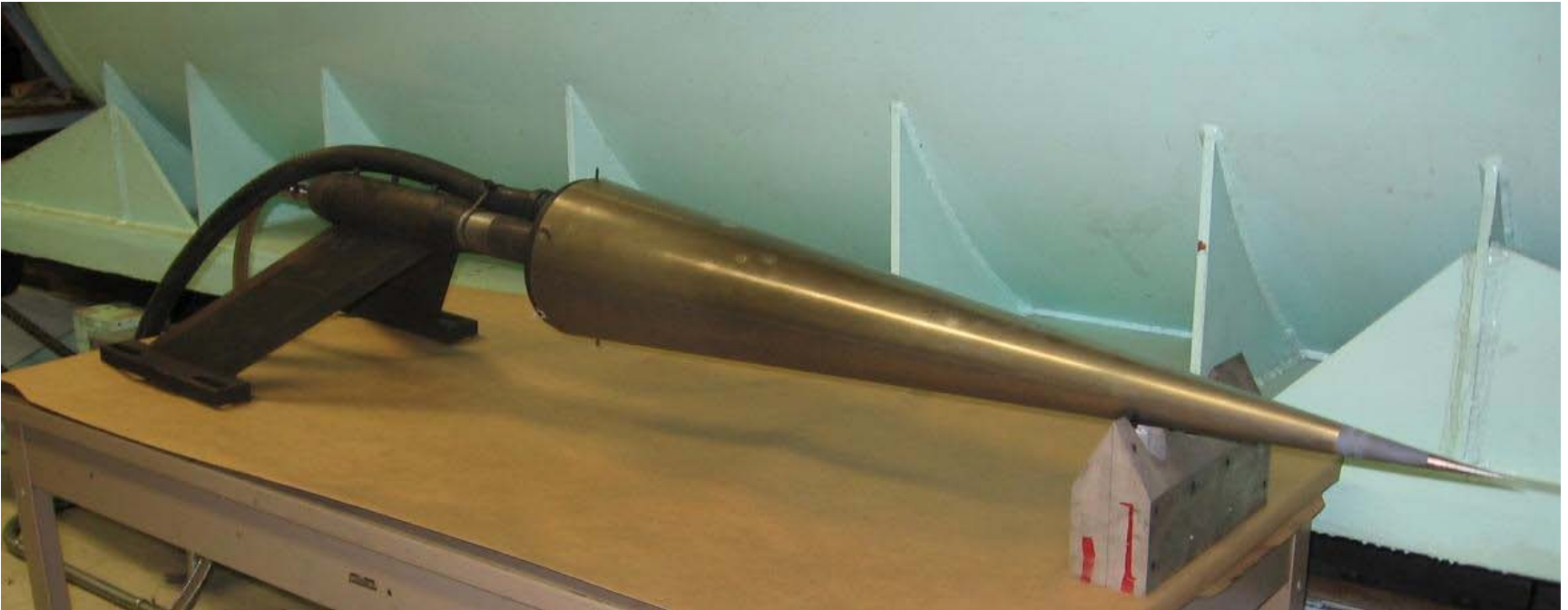
Injector section installed in ~1m long, 5-degree half angle cone
