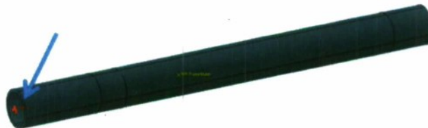
Figure 6 Encastre boundary condition applied to rigid body reference point to fix the gun tube
