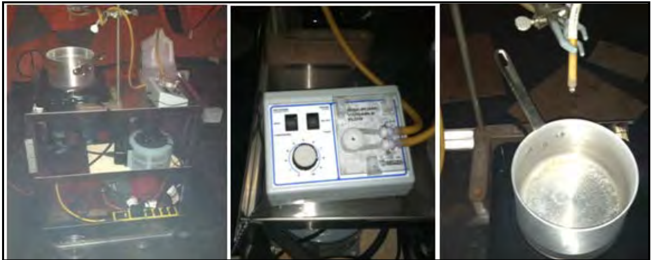
Figure 1. Typical condensation testing set-up.
