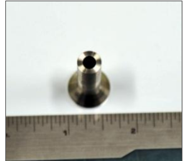
Fig10. Venturi Outlet (0.047") (AFRL/RZOP, 2011)
