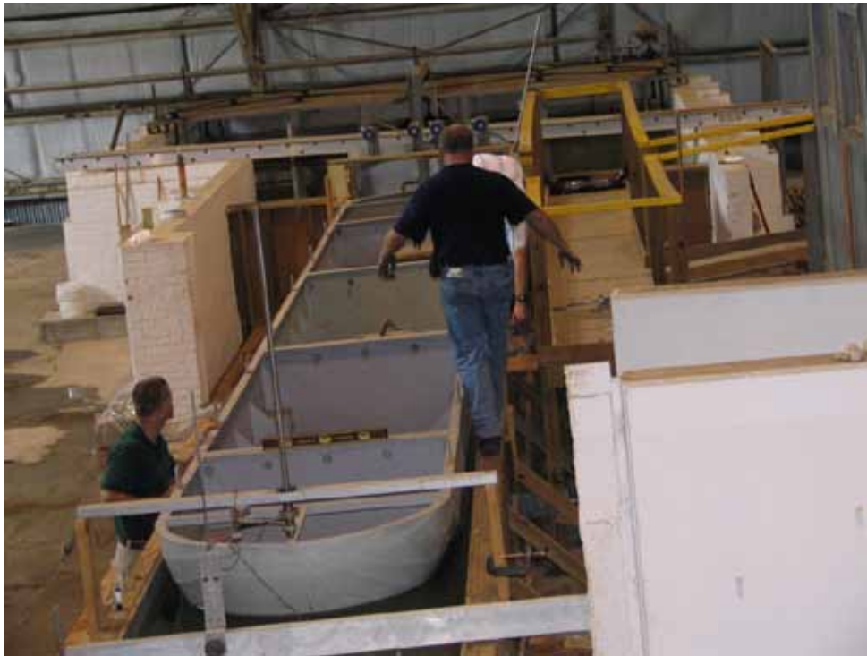
Figure 23. Ship in chamber for hawser force measurements with Type 15 Chamber Design.
