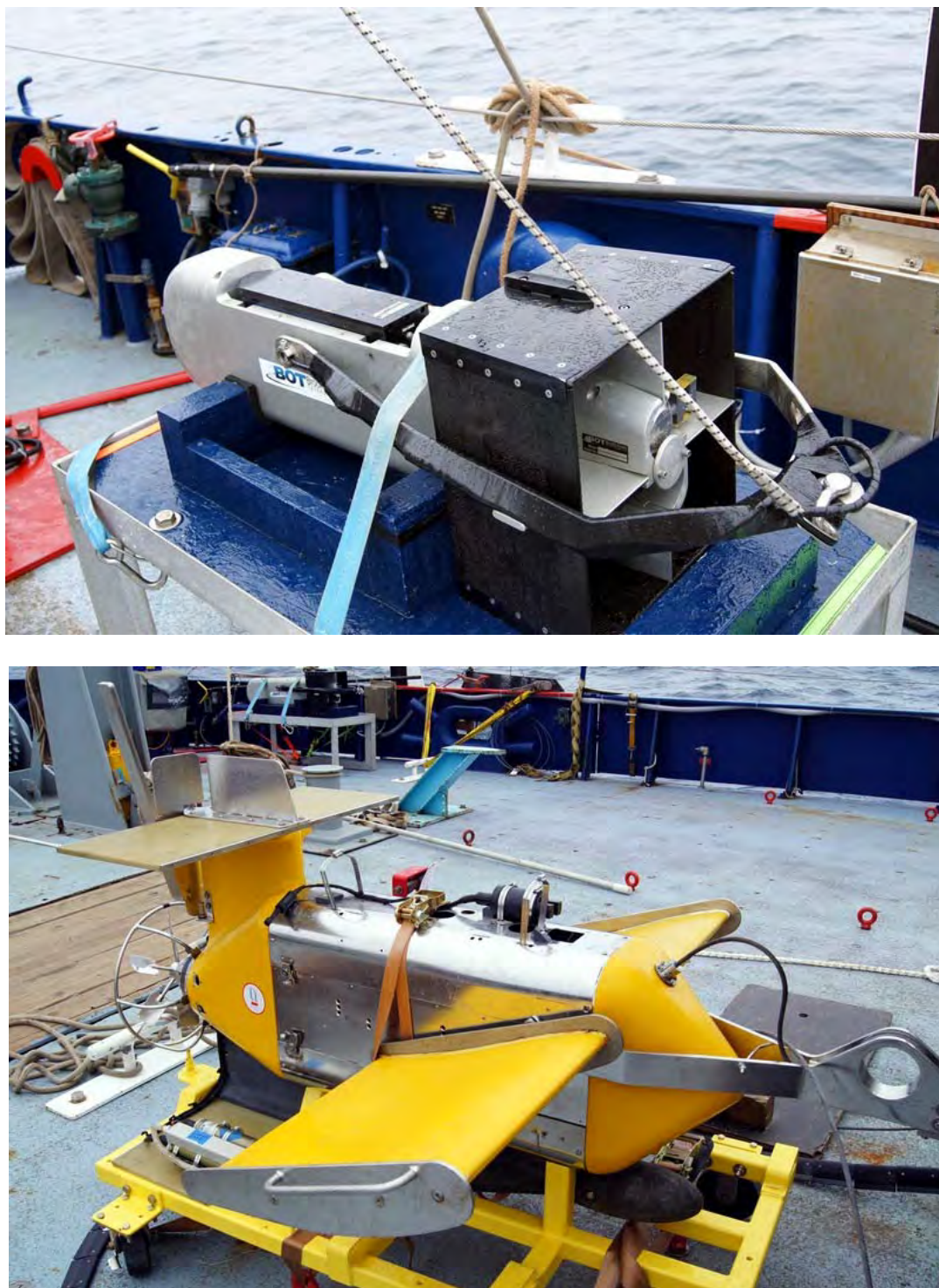
Fig. 10 The Moving Vehicle Profiler (MVP, upper photo) and the SeaSoar (lower photo) towed vehicles are considered as prospective platforms for deployments of the next generation, ALF In Situ instrument to be built during Y3 NOPP project research.
