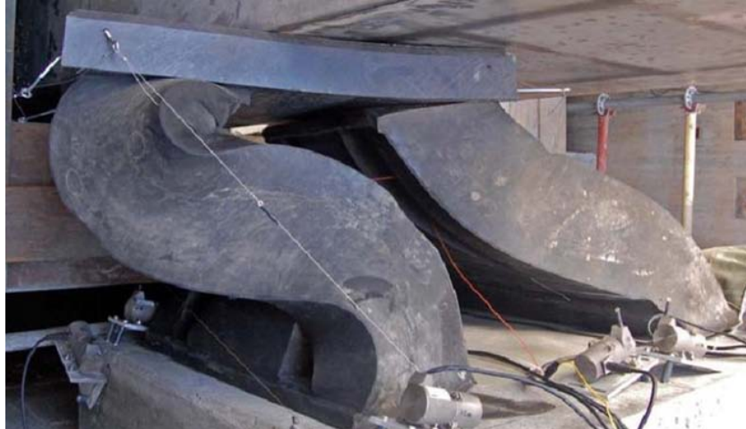
Figure 5-1. MHP Fender Sideway Collapse
