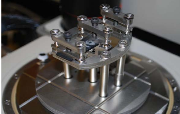
Figure 3-5. DMA Machine With a Test Specimen
