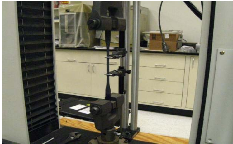
Figure 3-1. Tensile Testing of Rubber Specimens
