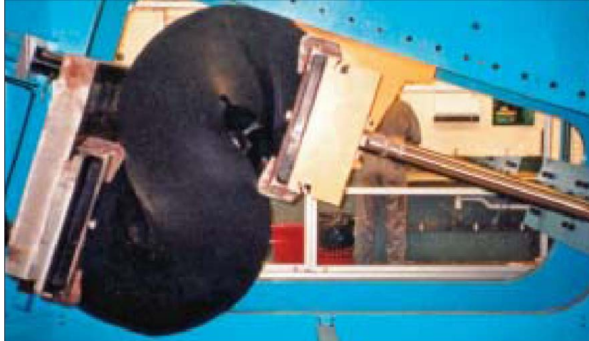
Figure 4-1. Single Element Deflection in a Test Structure
