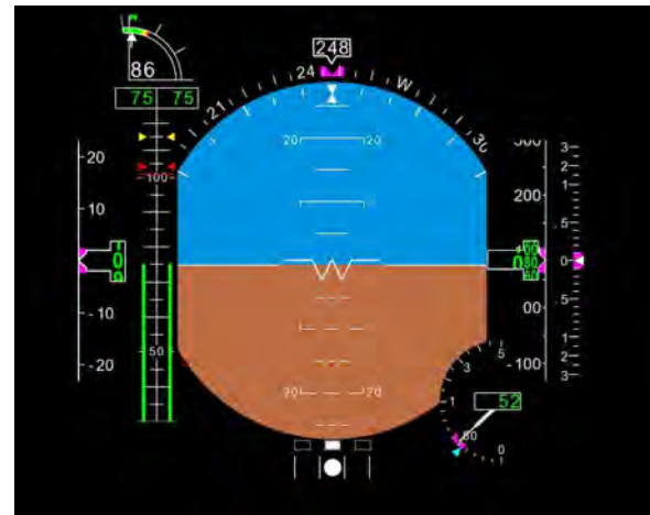
Figure 10. CAAS display with nacelle position indicator (top left)
