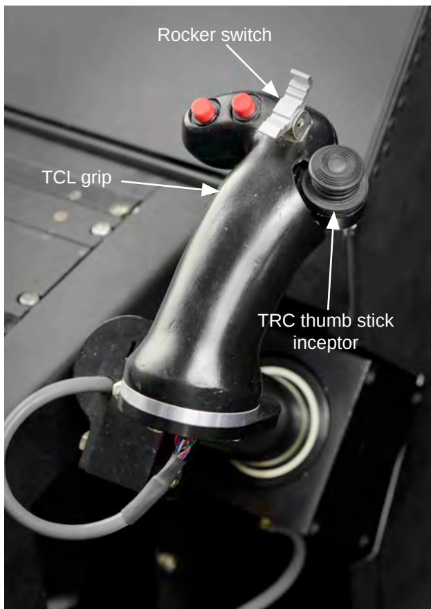
Figure 9. Thrust Control Lever Grip. Center rocker switch controls discrete nacelle movement. The thumb stick is a two-axis proportional controller. Used with TRC the stick provides an alternative to center stick inputs for longitudinal and lateral speed control. In ACAH, the thumb stick controls fore and aft nacelle rate, proportional to control displacement, up to a maximum of 7.5 deg/s.
