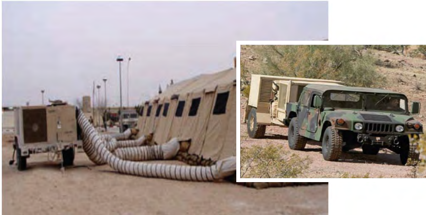
Combined heating, cooling and power generator used Iraq and Afghanistan, from CTO
