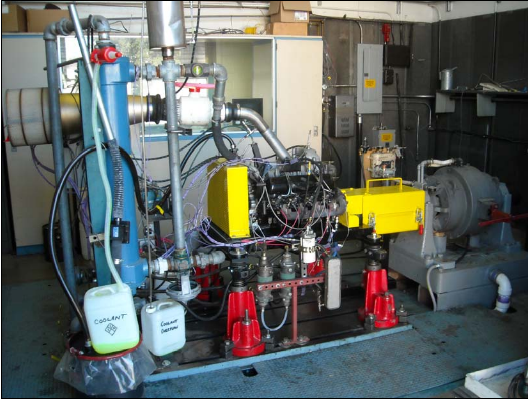
Figure 2 - GEP 6.5L(T) Test Cell Installation
