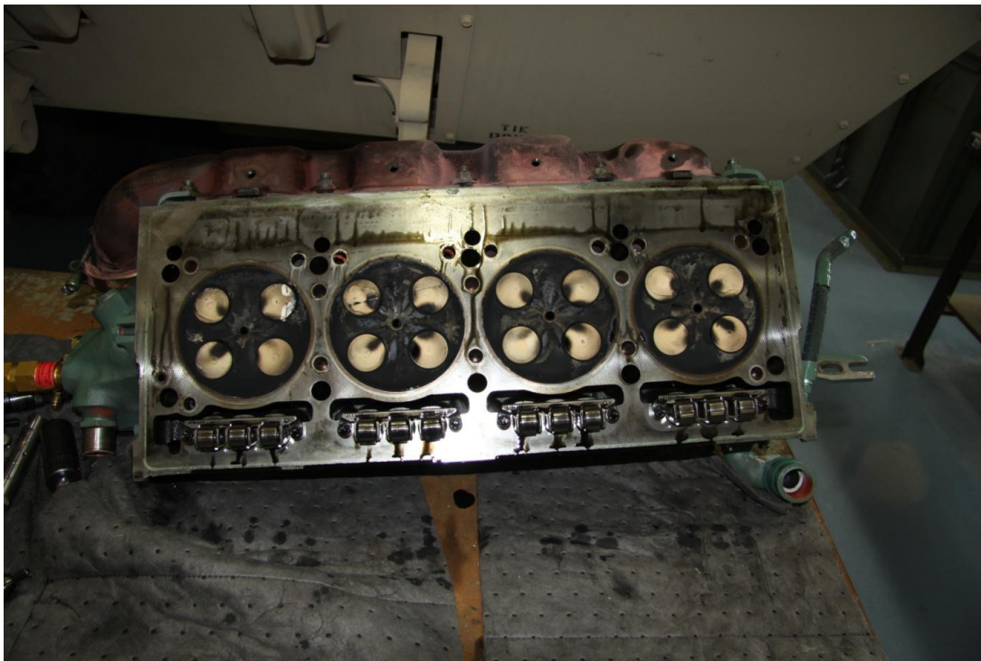
Figure 14. JP-8/FT engine cylinder heads 1,3,5,7 with debris build-up
