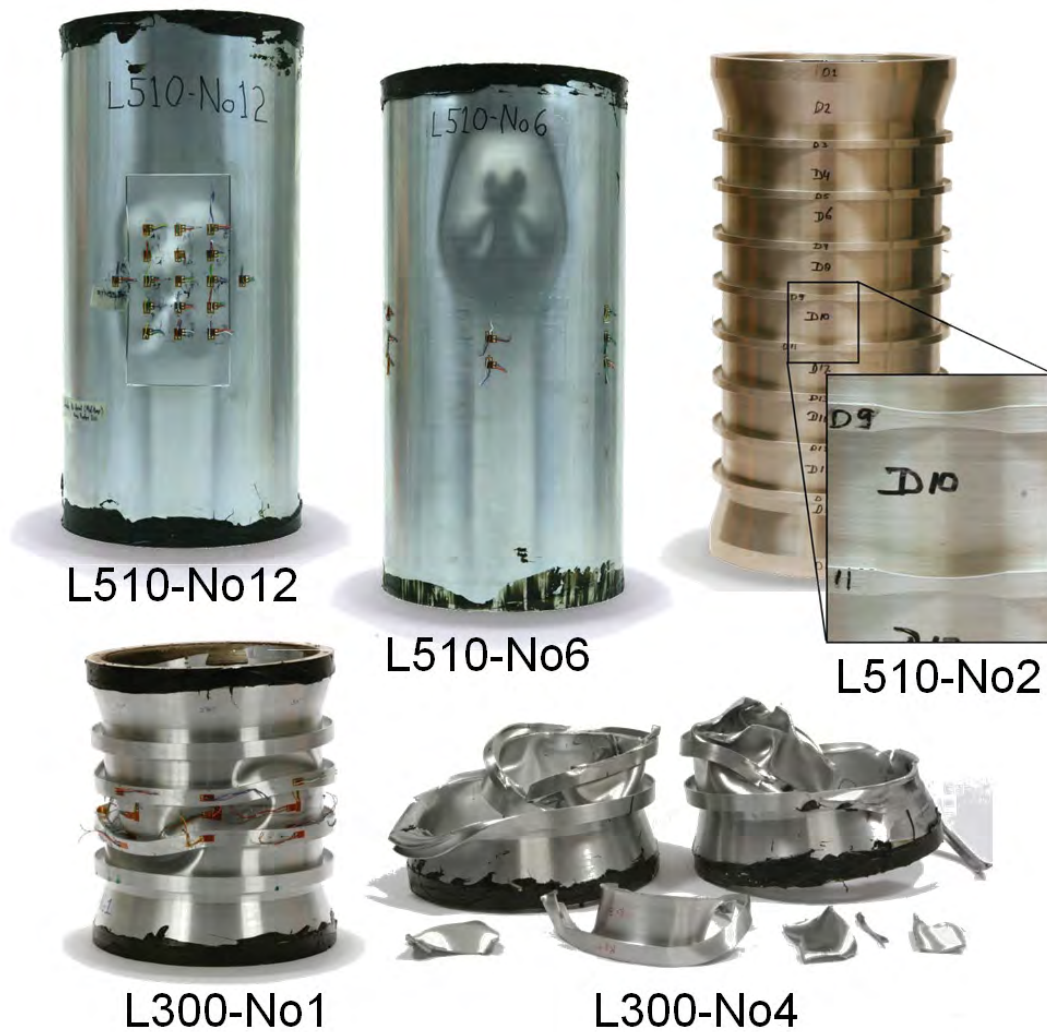
Figure 1: Some typical experimental models from previous phases of testing [10], before and after collapse testing. Clockwise from top-left: L510-No12, an internally-stiffened cylinder with a large patch of corrosion thinning, after volume-control testing; L510-No6, an intact internally-stiffened cylinder after volume-control testing, showing interframe dimples superimposed on an overall collapse mode; L510-No2, before testing, showing dog-bone stiffener corrosion at inset; L300-No4, a short cylinder with heavy stiffeners and a small patch of shell corrosion, showing the specimen after testing with a conventional apparatus; L300-No1, a short intact cylinder failing by interframe collapse, and showing the specimen after testing with a volume-control apparatus.
