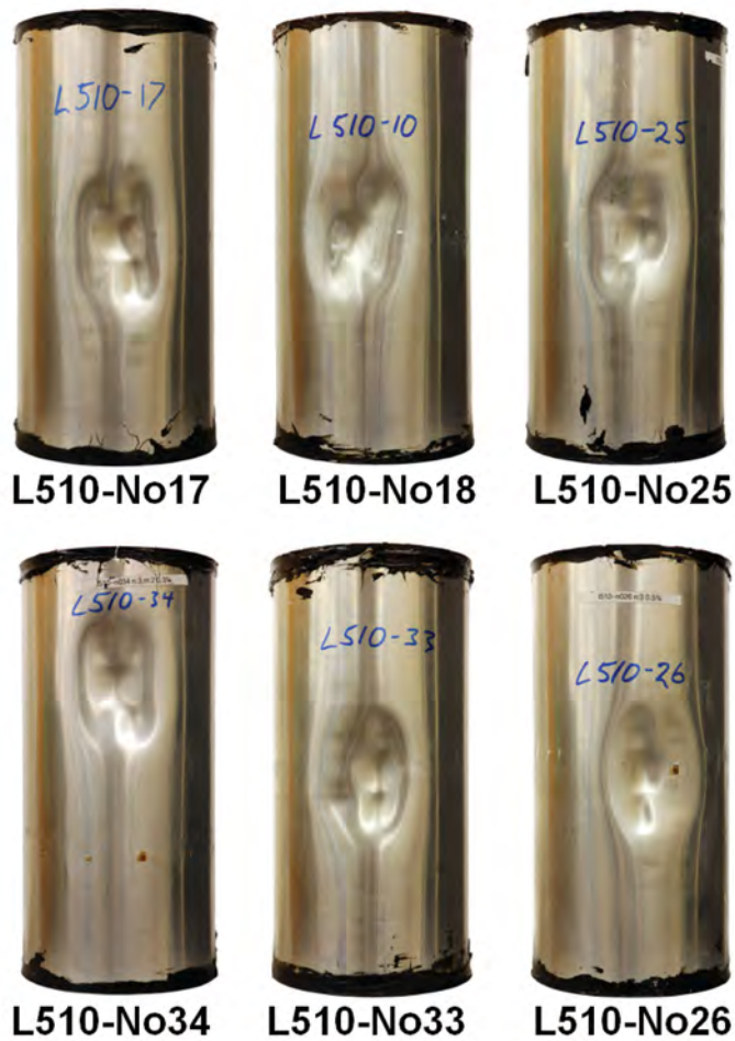
Figure 32: Phase 5 specimens, without artificial corrosion damage, after collapse testing. Clockwise from top-left: L510-No17 and L510-No18, both with 0.3% OOC in n=3 and m=1 circumferential and axial modes, respectively; L510-No25, L510-No26 and L510-No33, all with 0.5% OOC in n=3 and m=1 circumferential and axial modes, respectively; and L510-No34, with 0.3% OOC in n=3 and m=2 circumferential and axial modes, respectively.
