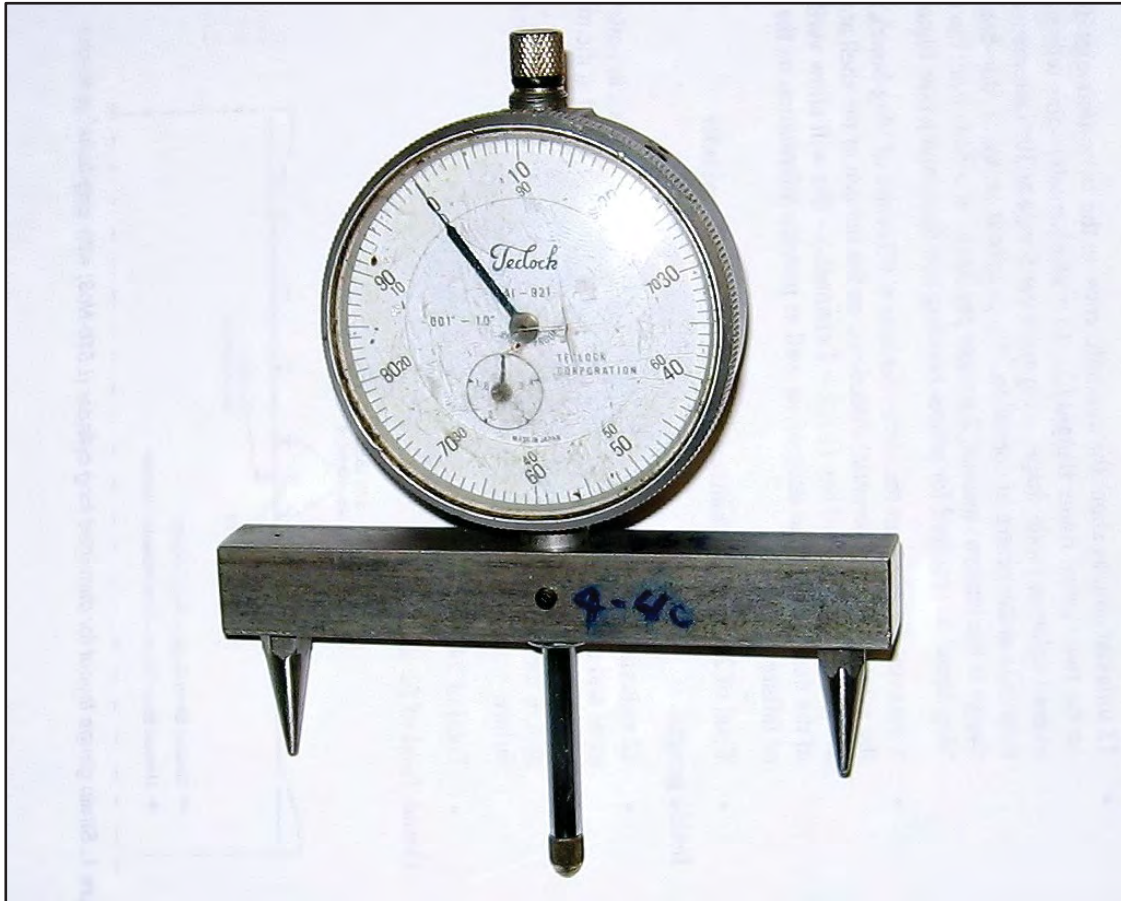
Figure 6: Chord gauge device used to measure the out-of-circularity of Phase 5 cylinder specimens.
