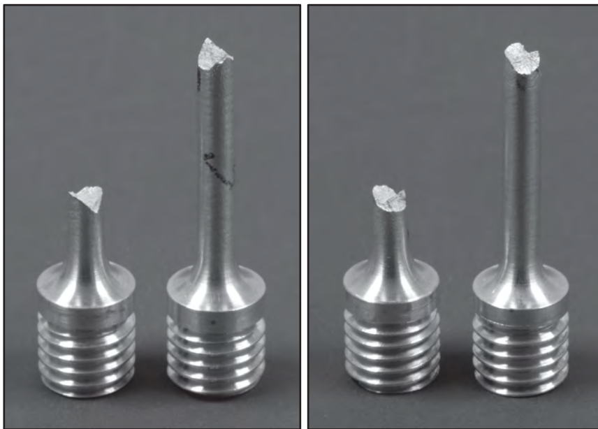
Figure 25: Typical post-testing configuration of under-sized tensile coupons, showing coupons taken from Phase 2 cylinders [2] constructed from AA-6082-T6 tubing.
