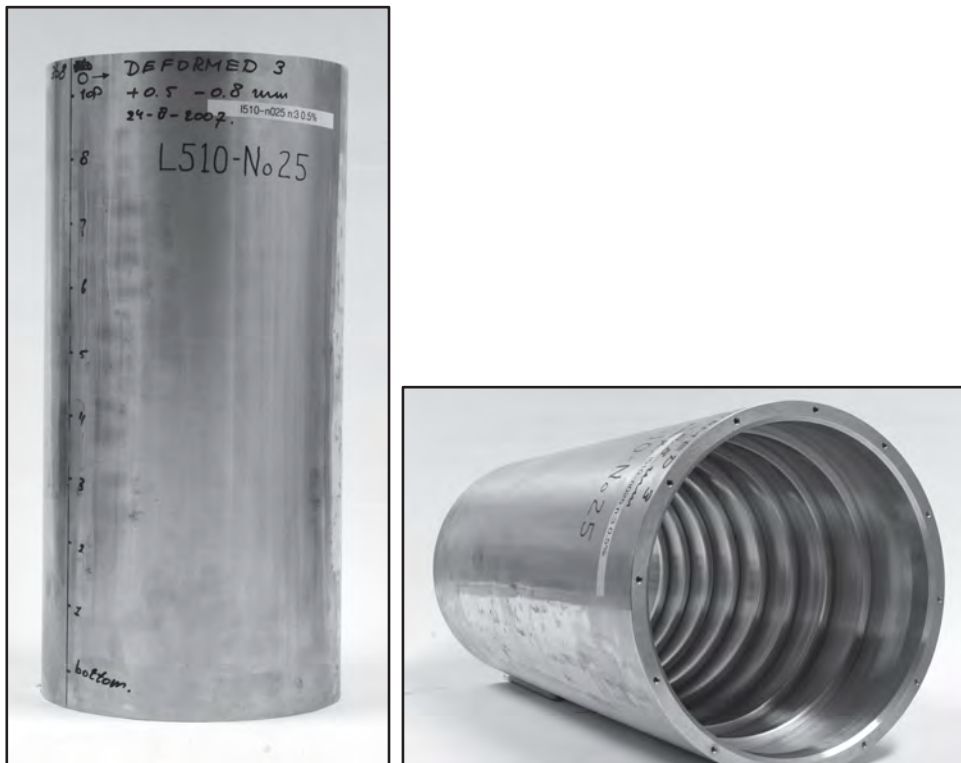
Figure 2: Photographs of a typical intact specimen, L510-No25, before testing.
