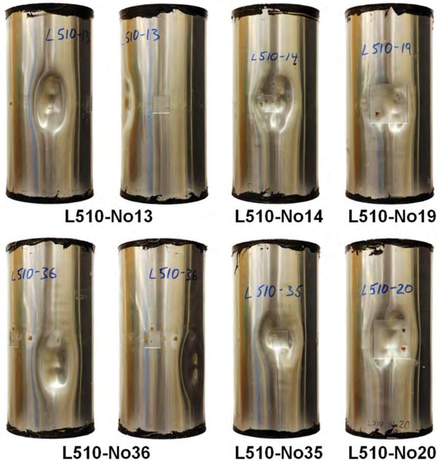
Figure 57: Phase 6 specimens, with artificial corrosion damage and 0.5% OOC in n=3 , m=1 mode, after collapse testing. Clockwise from top-left: L510-No13, with a 42x42x0.6 mm, out-of-phase corrosion patch, showing photographs of the collapse location and the corrosion patch location relative to the collapse site; L510-No14, with a 42x42x0.6 mm, in-phase corrosion patch; L510-No19 and L510-No20, with 100x100x0.4 mm, in-phase corrosion patches; L510-No35, with a 42x42x0.6 mm, in-phase corrosion patch; and L510-No36, with a 42x42x0.6 mm, out-of-phase corrosion patch, showing photographs of the corrosion patch location relative to the collapse site and the collapse location itself.
