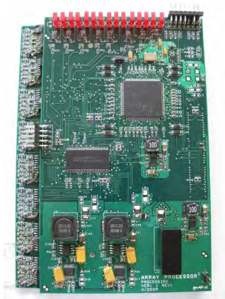
Figure D.2 The acquisition and processing unit.
