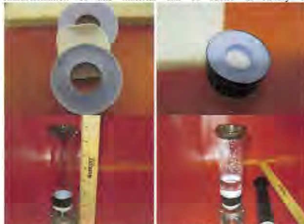
Figure 1. Experimental setup to determine fabric breakthrough pressure.
