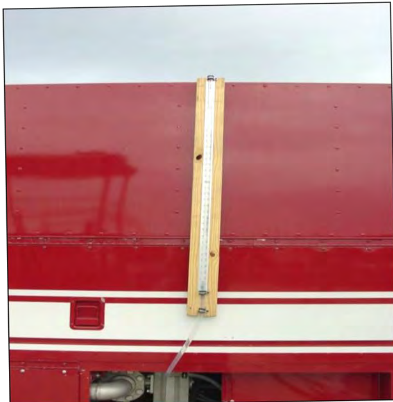
Figure 4. Manometer for Tank Level Measurement
