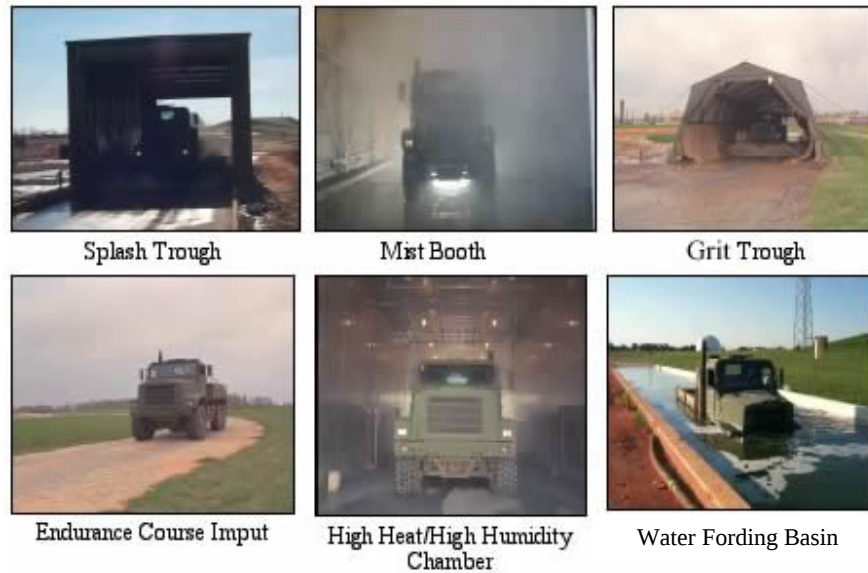
Figure 27. Accelerated Corrosion Complex.
