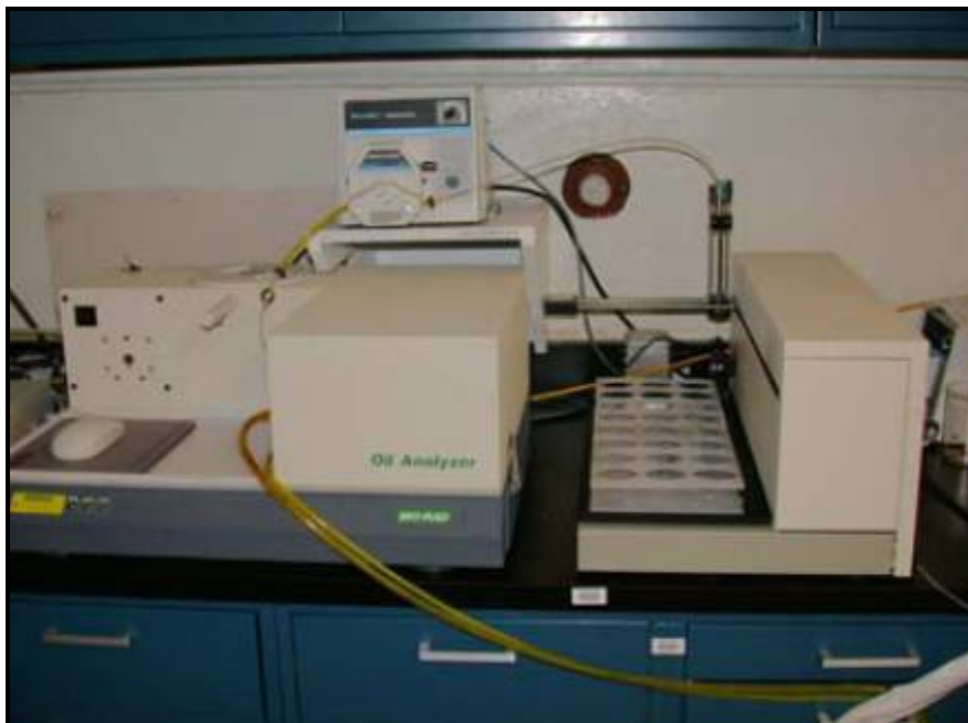
Figure 184. Advanced oil analyzer platform Fourier Transform Infrared Spectrometer used for molecular analysis of lubricants and hydraulic fluids.
