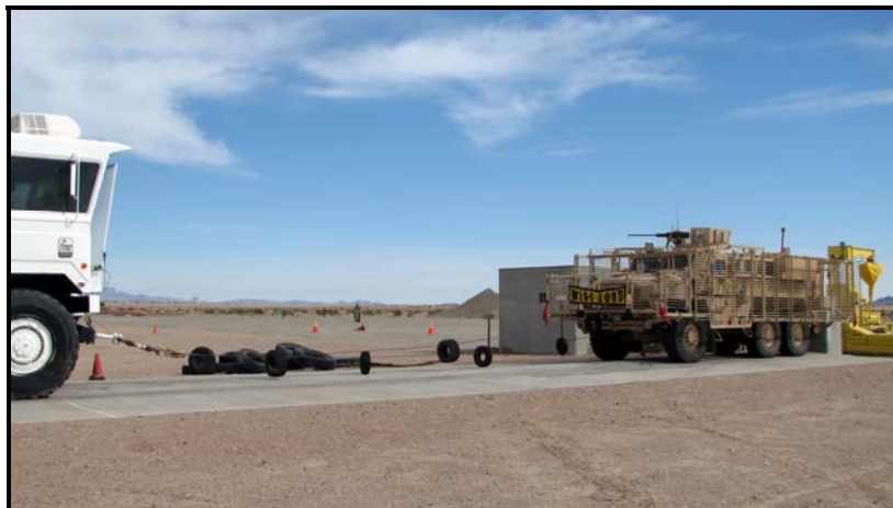
Figure 155. Vehicle undergoing winch testing.
