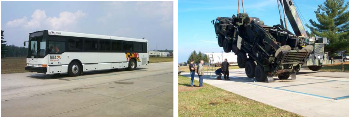
Figure 91. Vehicles on platform scales.
