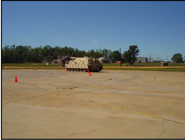
Figure 62. Measurement of vehicle turning diameter on the Munson Turning Circle.
