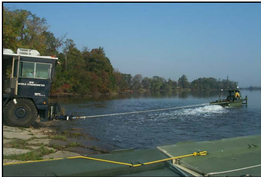
Figure 35. Bollard pull using mobile field dynamometer.
