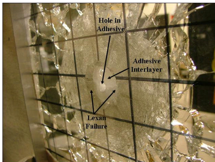
Figure 23. Lexan failure on rear side of 0.22-cal bonded glass targets.
