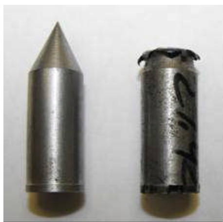
Figure 5. Photograph of 0.50-cal bullet (Rc30) showing considerable nose erosion and mushrooming.
