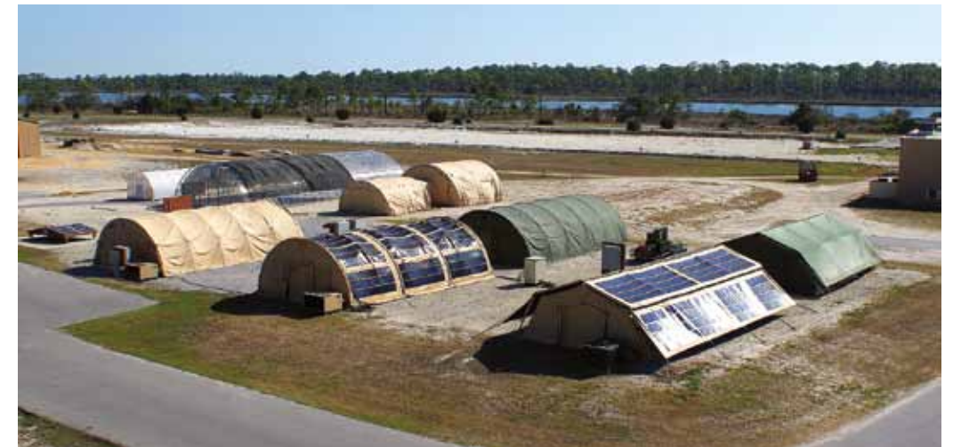
Deployable solar power is tested and evaluated at the Air Force Research Laboratory's Renewable Energy Tent City at Tyndall, AFB, Fla. (U.S. Air Force photo)
