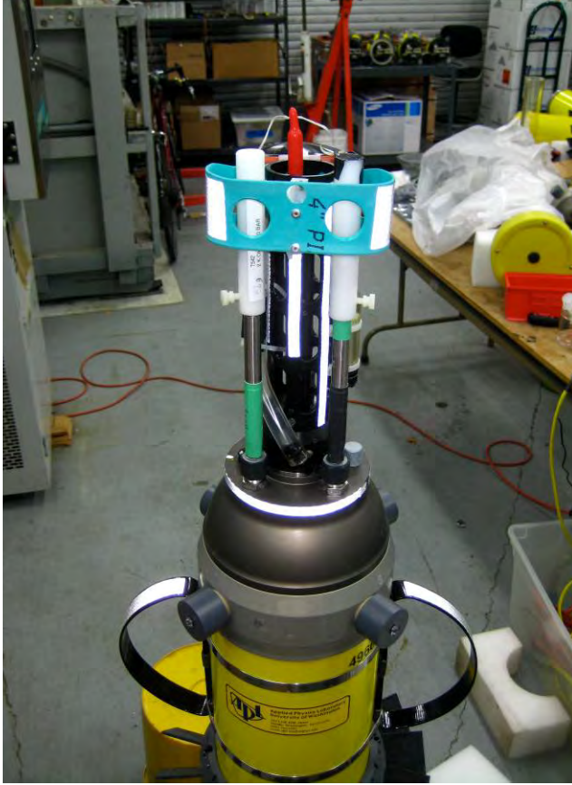
Fig. 1(a): EM-APEX float with Chi sensors with white plastic covers behind blue guard.
