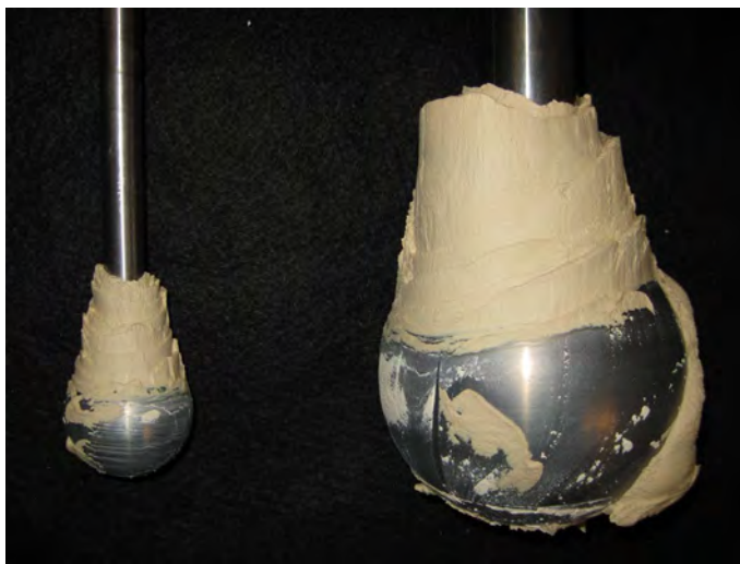
Figure 2: Photograph of soil flow mechanism around mini-ball and standard ball penetrometers after extraction from laboratory clay specimen.
