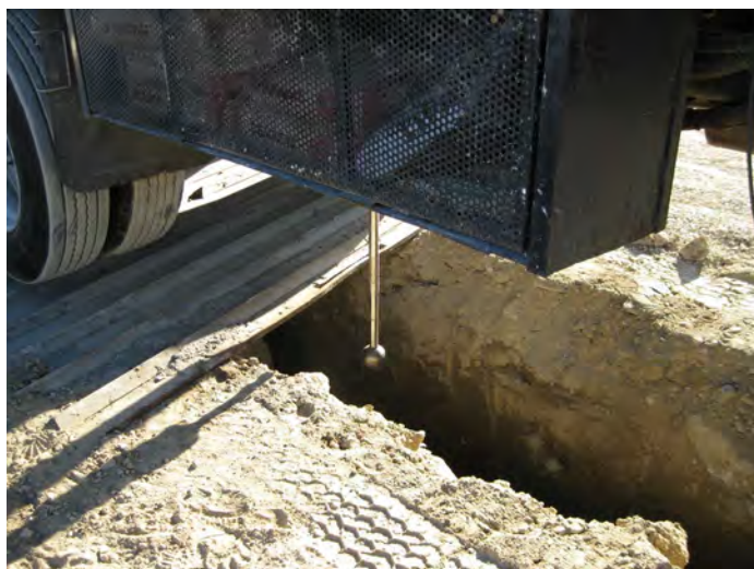
Figure 3: Photograph during preparation of ball penetrometer for testing in soft mine tailings at quarry site in Irwindale, California.
