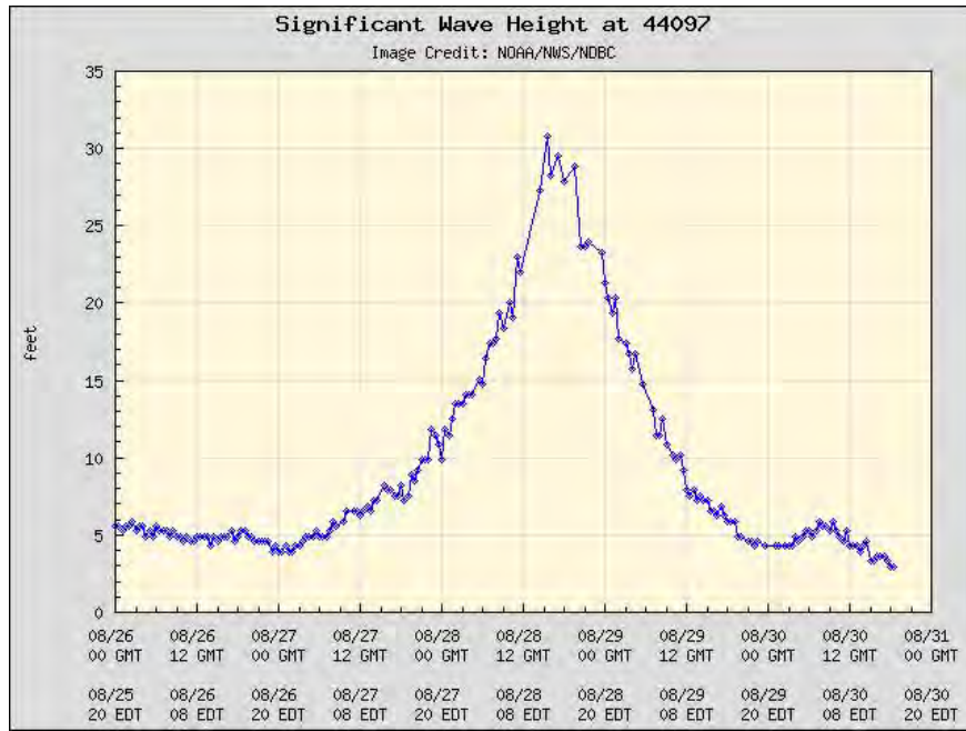
Figure 5. Significant Wave Heights from NOAA Buoy 44097 offshore of Block Island in 50m water depth during Hurricane Irene
