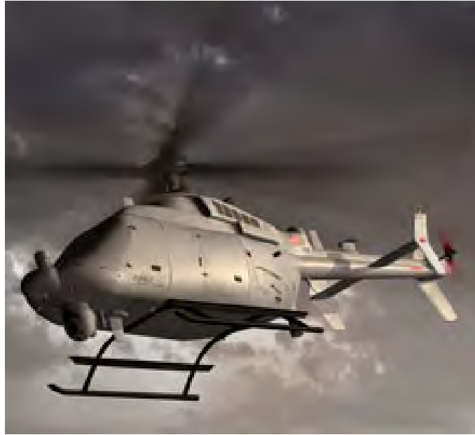
Figure 5. Fire-X UAS based on the Bell Helicopter 407 airframe and FireScout flight control system.
