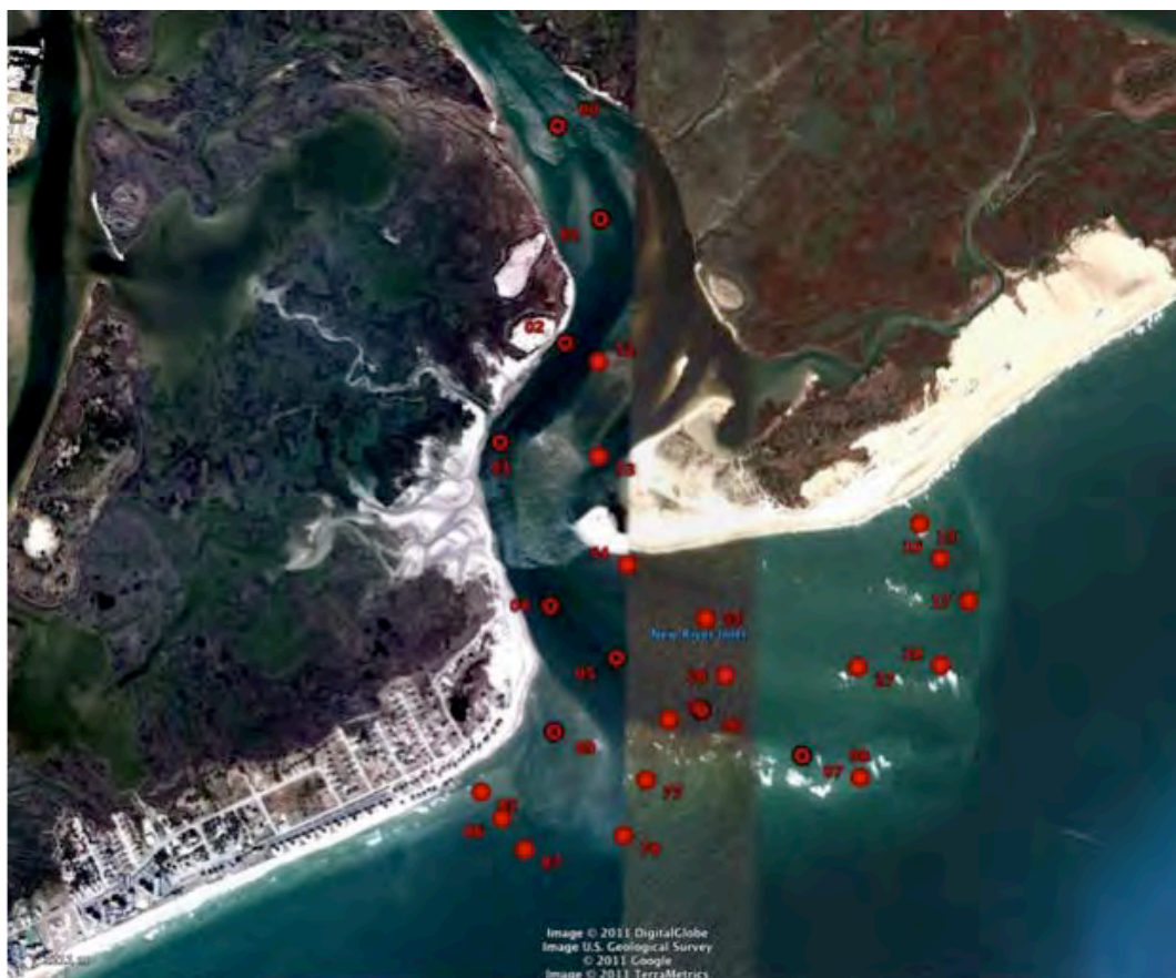
Figure 1. Array of in situ sensors planned for New River Inlet, spring 2012. Solid red circles are colocated pressure sensors and acoustic Doppler velocimeters. Black and red circles are colocated pressure gages and acoustic Doppler profiling current meters. CTDs will be colocated with some of the sensors. Bathymetry will be surveyed pre and post deployment, and weekly during the experiment [Instruments are located across the ebb shoal and about 2 km up the river].
