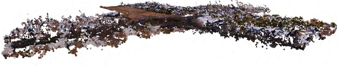
Figure 56. Substantially improvement in the RMSDE accuracy was observed when two orthogonal passes were combined. Furthermore note the substantial noise in the non-overlapping areas and reconstruction fidelity contained within the overlapping area.
