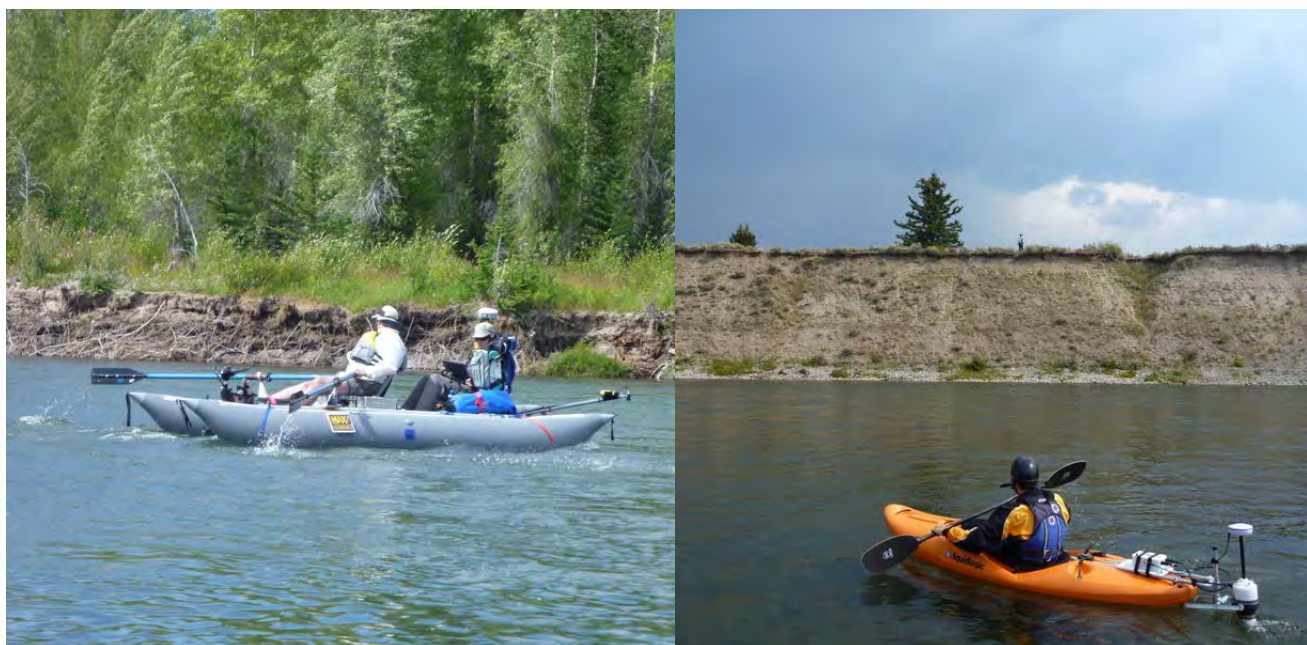
Figure 1. (a) Research cataraft instrumented with an echo sounder, RTK GPS, turbidity sensor, and spectroradiometer deployed along the Snake River. Here, we are measuring reflectance via the fore-optic mounted on the boom extending from the rear of the vessel. (b) Kayak with acoustic Doppler current profiler used to measure vertical profiles of flow velocity along the Snake River.
