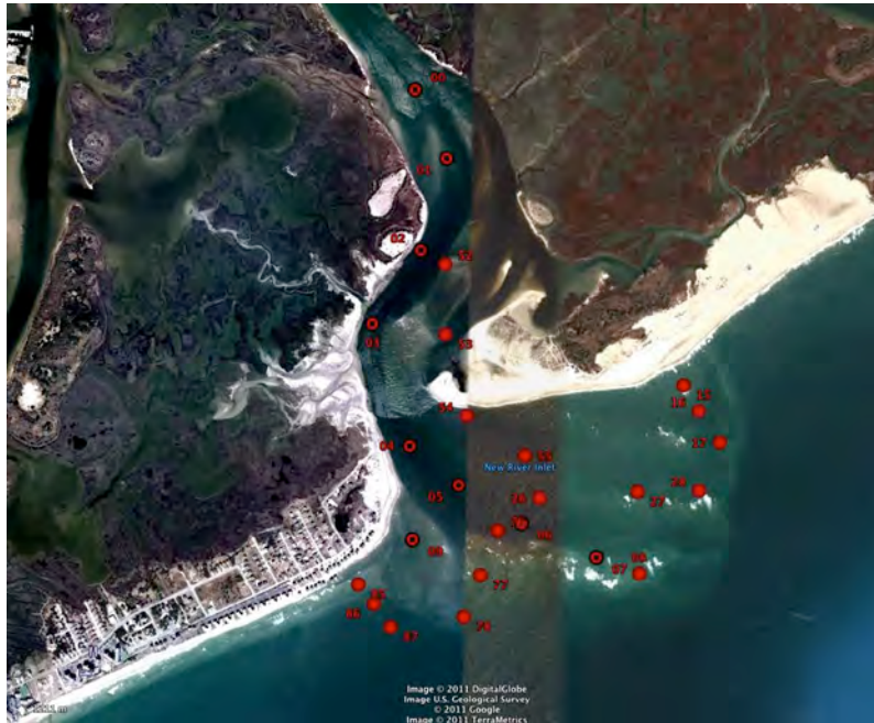
Figure F1. Array of in situ sensors planned for New River Inlet, spring 2012. Solid red circles are colocated pressure sensors and acoustic Doppler velocimeters. Black and red circles are colocated pressure gages and acoustic Doppler profiling current meters. CTDs will be colocated with some of the sensors. Bathymetry will be surveyed pre and post deployment, and weekly during the experiment.
