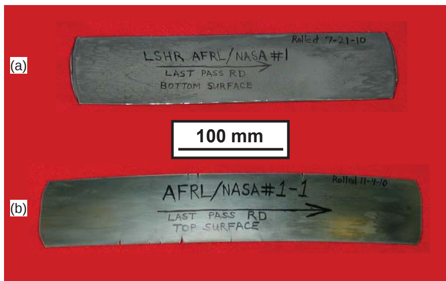
Figure 2. Macrographs of LSHR produced by near-conventional hot pack rolling: (a) Sheet and (b) foil.
