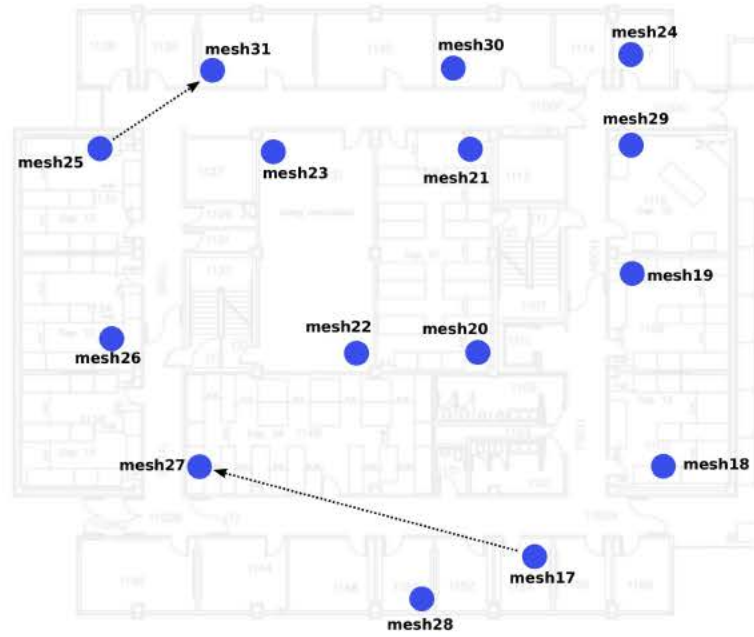
Figure 7: Wireless mesh topology
