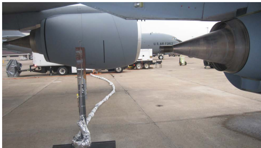
Figure 4. Schematic (upper panel) and picture (lower panel) of the sampling rake used for the tests at the Pittsburgh International Airport. The center inlet of the rake was aligned with the oil vent, which is the cone-shaped piece protruding from the back of the engine.
