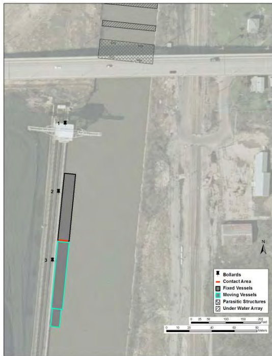
Figure 5. Sparking potential testing scenario for a tow with barges in series, 5 February 2011.
