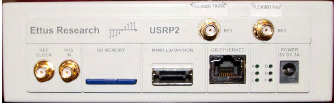
Figure 3.7: Front view of a USRP2.
