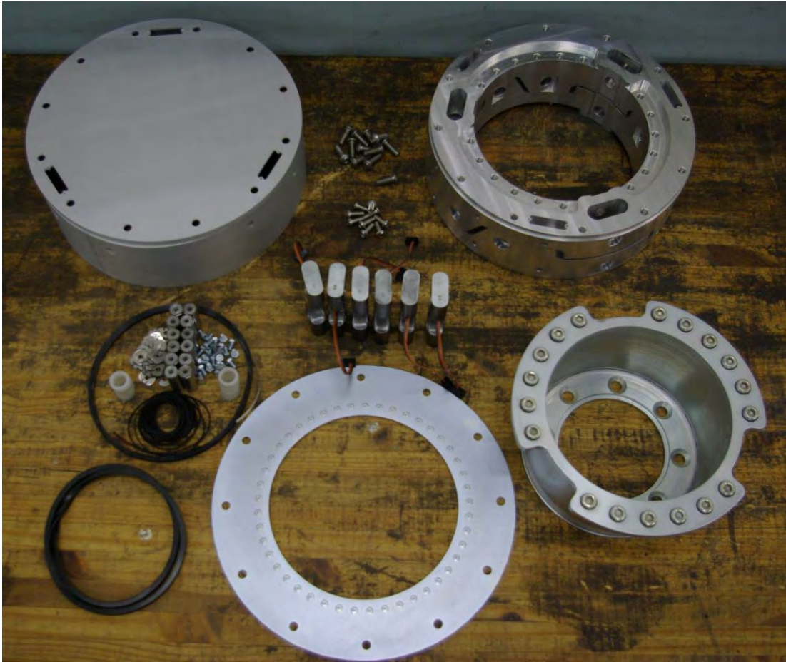
Figure 6 - Components of a wheel force transducer
