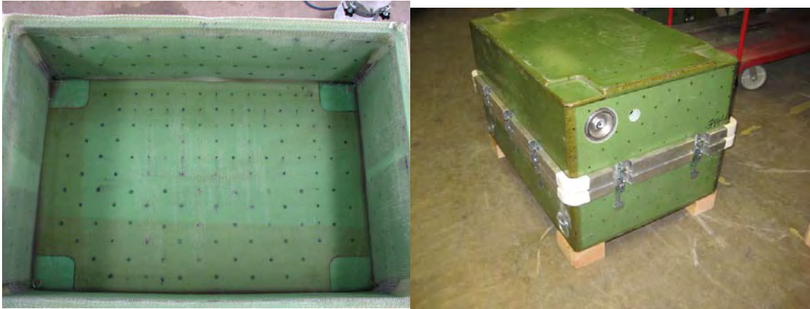
Figure 8. Photograph of the inside of completed laboratory-demonstrated HMMWV transmission container (left) and assembled FAVE HMMWV transmission container manufactured by SMC (right).
