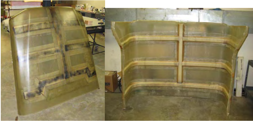
Figure 10. Topside of FAVE-L-HT-RDX M35A3 hood (left) manufactured by SMC and the underside of FAVE-O-HT-RDX M939 hood (right) manufactured by CCM.
