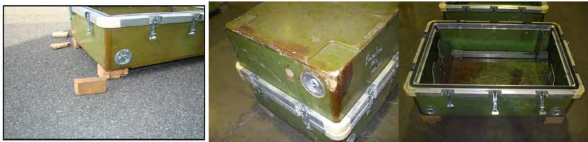
Figure 9. Photograph showing the broken wooden feet after loose cargo testing (left). Evidence of corner impact—local crushing but still holding together (middle). Transmission fluid bled into core (right).
