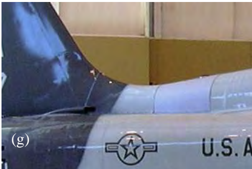
Figure 2. This program demonstrated/validated low HAP VE resin composites for (a) HMMWV ballistic hardtop; (b) an HMMWV transmission container; 1-2 types of composite replacement hoods, including; (c) M939, (d) M35A3, or (e) HMMWV; (f) MCM rudder; (g) T-38 dorsal cover; and (h) F-22 canopy cover.
