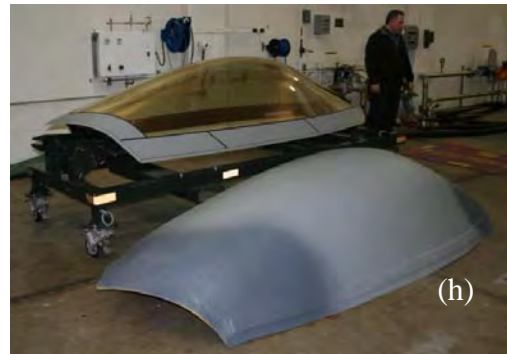
Figure 2. This program demonstrated/validated low HAP VE resin composites for (a) HMMWV ballistic hardtop; (b) an HMMWV transmission container; 1-2 types of composite replacement hoods, including; (c) M939, (d) M35A3, or (e) HMMWV; (f) MCM rudder; (g) T-38 dorsal cover; and (h) F-22 canopy cover.
