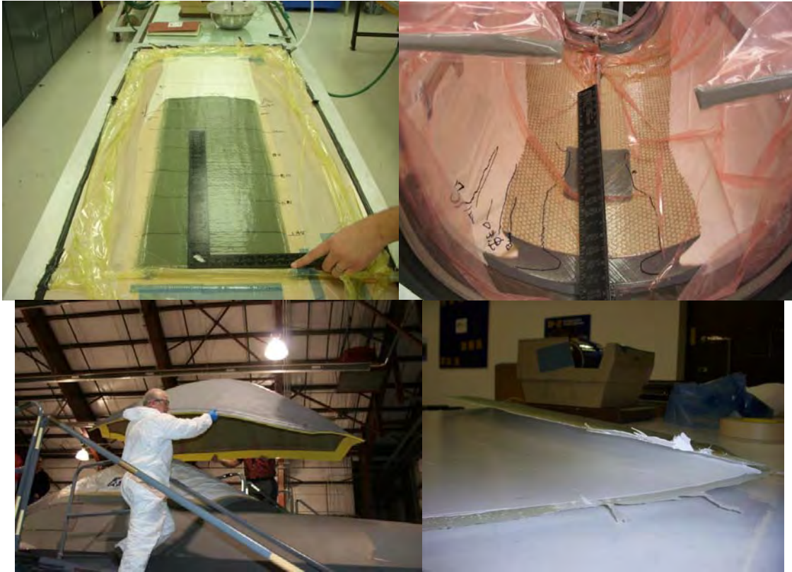
Figure 6. Top left - splash mold resin flow test. Top right - failed attempt to infuse T-38 dorsal cover with FAVE-L. Bottom left - final F-22 canopy cover being fit tested on an F-22. Bottom right - splash mold, after removal from aircraft surface.
