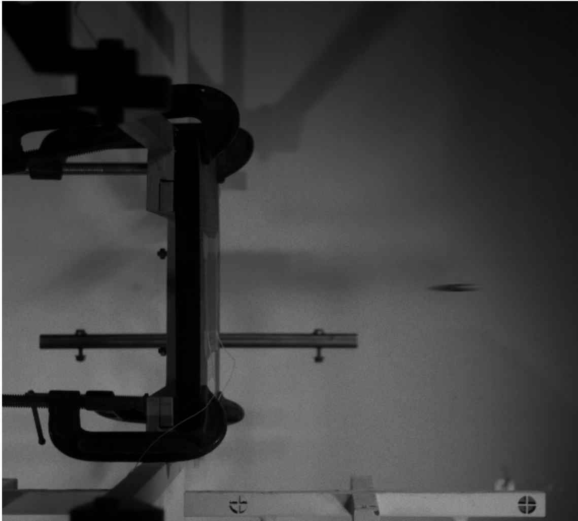
Figure 4.16. Side View of the Projectile Prior to Impact
