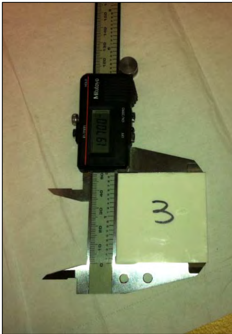
Figure 3.16. Measuring the Dimensions of Ceramic Coupon #3
