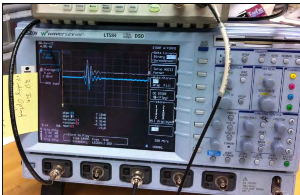
Figure 3.21. Oscilloscope Used to Capture Output Wave Propagations
