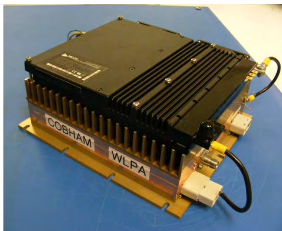
Figure 9. Photo of Completed WLPA Module [5]
