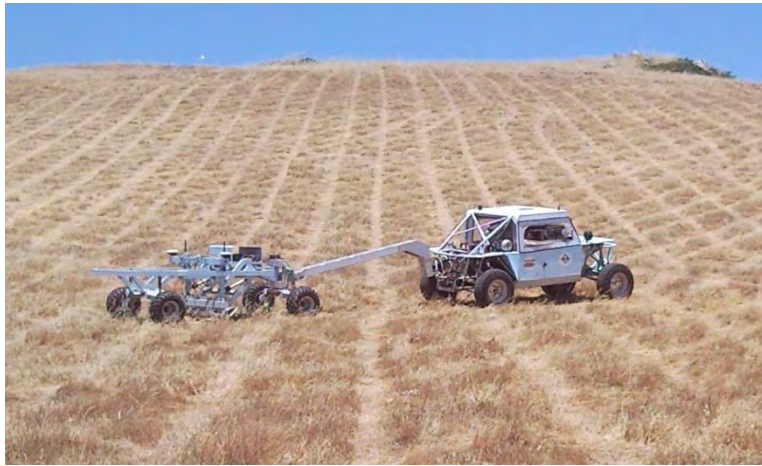
Figure 1 – MTADS tow vehicle and magnetometer array.
