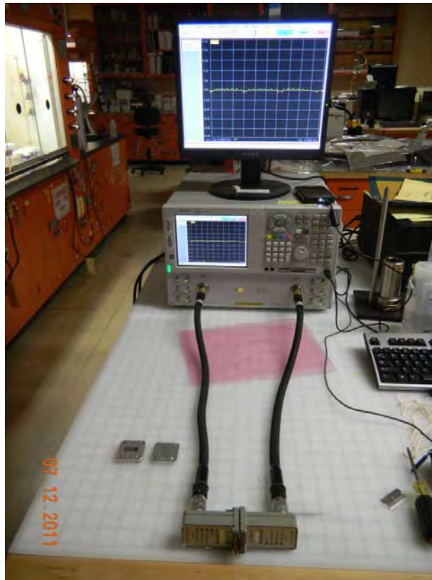
Figure 22. Network Analyzer used to measure EMI-SE.
