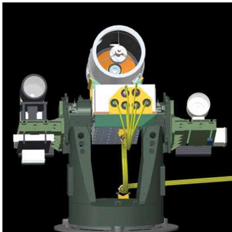
Figure 4. LaWS Beam Director Assembly Model
