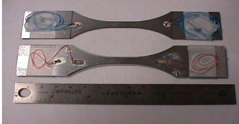
Figure 24: Bonded Sensors on Dogbone Specimens
