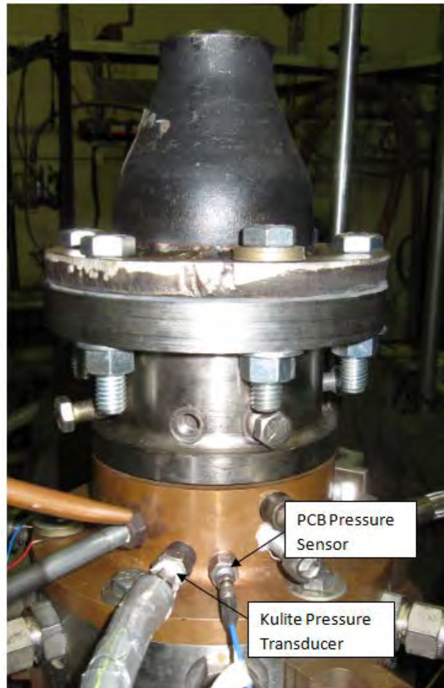
Figure 10. Experimental setup for 1.5 in. convergent nozzle on RDE
