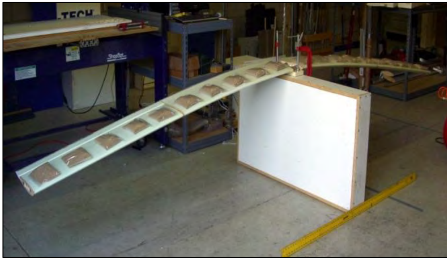
Figure 16: CLMax Wing Loading Tests (15-ft Wingspan)
