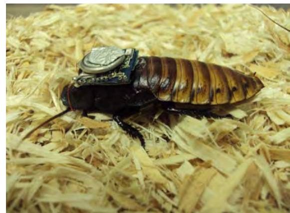
Figure 3. Mounting of custom RF board on Madagascar "Hissing" Cockroach ( Gromphadorhina portentosa ).
