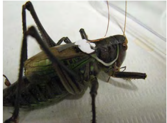
Figure 4. A photo showing the attachment of an IPMC strip to katydid's back using Whiteout as the adhesive.
