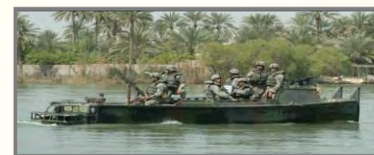
Bridge Erection Boat (L)
