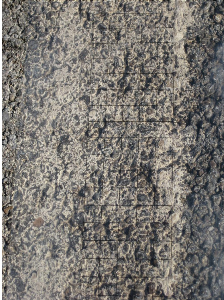
Figure 9: Transparent Grid Used for Measuring Coverage
