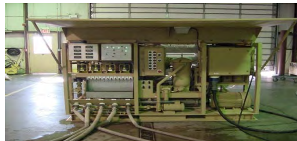
Reverse Osmosis Water Purification Unit (ROWPU)
