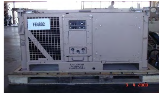
Environmental Control Unit (ECU) -9
