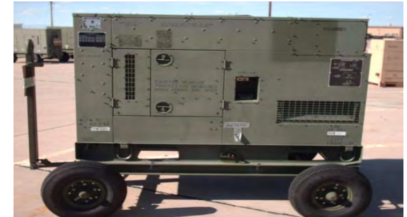
Mobile Electric Power (MEP) 805
