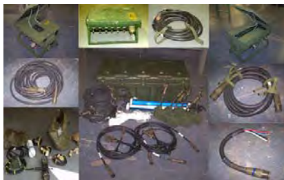
Power Distribution Illumination System Electrical (PDISE)
